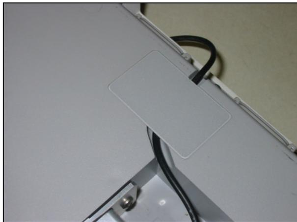
This image shows the unit with the cable routed through the channel.
