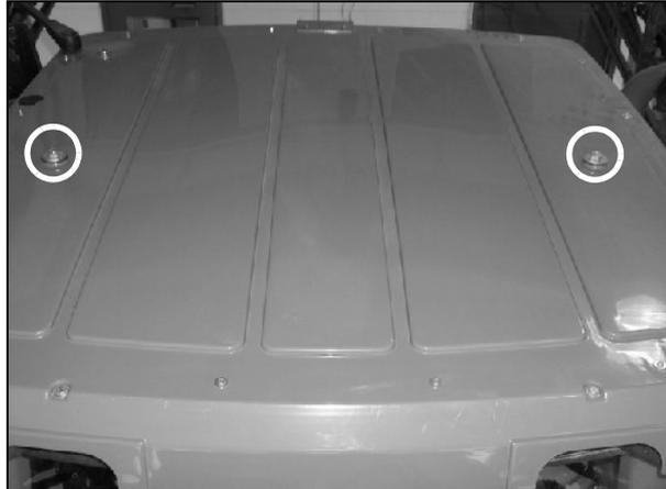
If a light bracket already occupies the roof studs, mount the spar directly onto the light bracket.
