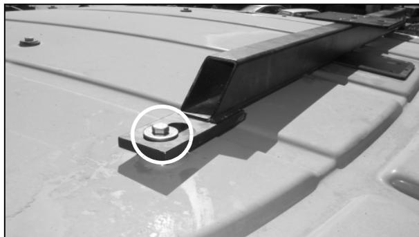
If you use the light bracket, drill two holes to match the spar width.
