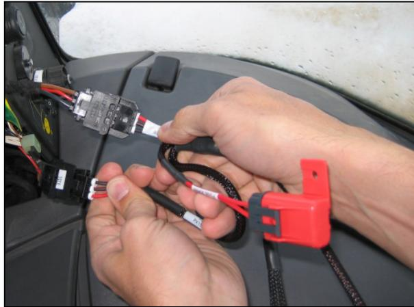
If the vehicle is an early model, use the power adapter supplied and route the ring terminal ends to the power posts located in the fuse compartment, and then connect the +12V lead to the +Bat post X12 and the Ground lead to the Ground post.
