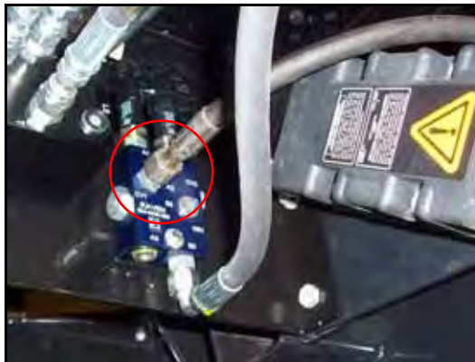
FIGURE 7. Machine's Left Steering Hose Installed on Flow Switch
