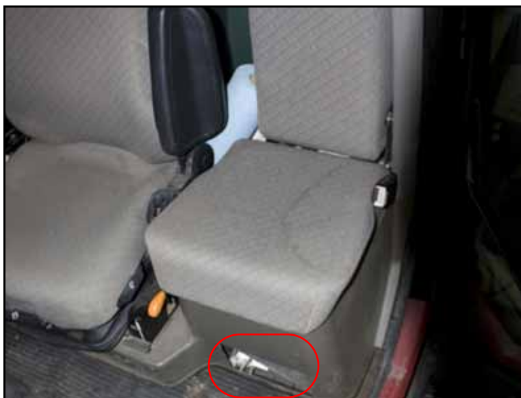
FIGURE 1. SmarTrax Node Mounting Location
