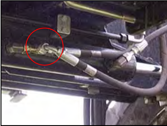
FIGURE 9. Second Left Steering Hose Installed
