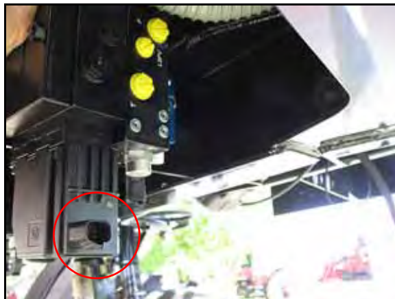
FIGURE 16. VALVE Harness Connection
