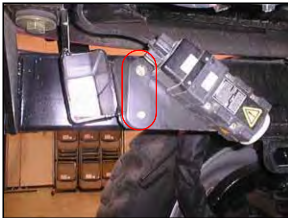
FIGURE 4. Machine's Radar Bracket Bolts
