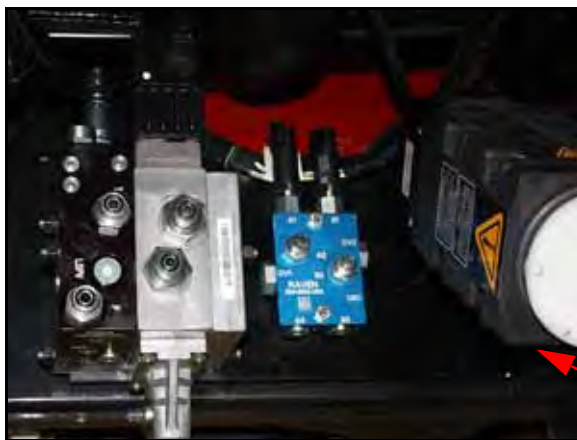
FIGURE 5. Valve Mounting Bracket Installed
