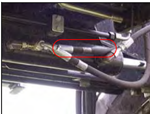
FIGURE 8. Left Steering Hose Installed
