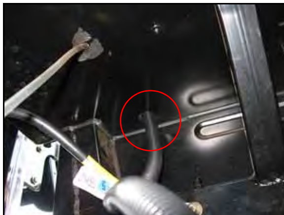
FIGURE 15. Valve Harness Routed into Cab
