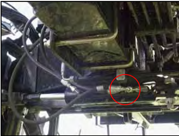
FIGURE 10. Right Steering Hose Installed
