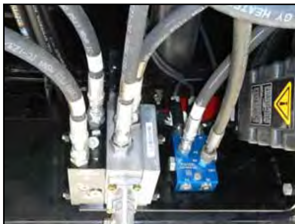
FIGURE 17. Valve Harness Connected to Flow Switch
