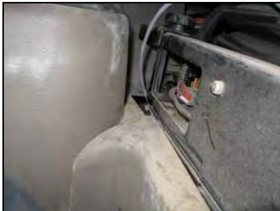
FIGURE 7. DGPS OUT Connector Routed Under Operator's Seat
