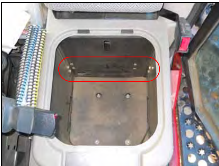
FIGURE 2. Bolts to be Removed
