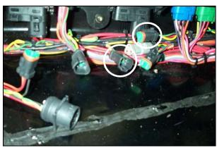
Ensure that the CAN cable has been connected together. Identify the two connectors by the attached wires:
